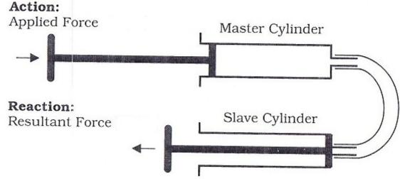
Fill the system by first inserting the master cylinder tip into a filled beaker and drawing back the plunger (A). Next attach the piece of tubing and fill it with water by forcing the piston to expel water (B). Finally, attach the other syringe, the slave, to the other end of the tube (C). Make sure the piston is completely pushed in before connecting the tube!
